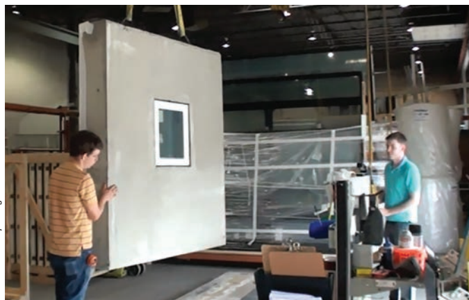
A full-scale ICF test module is craned into position at testing facility by RDH engineers.
